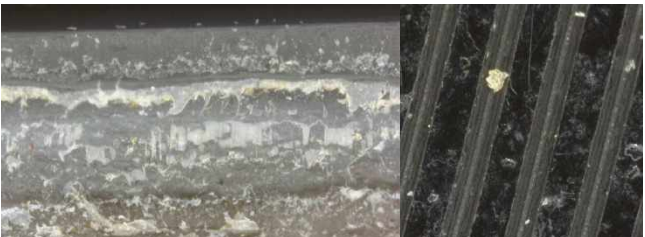
Decelith flexible, Radio-Genève, Y272, 1942. Right: Stratigraphy, cross section. Left: groove walls striations. USB micrograph, 250x
