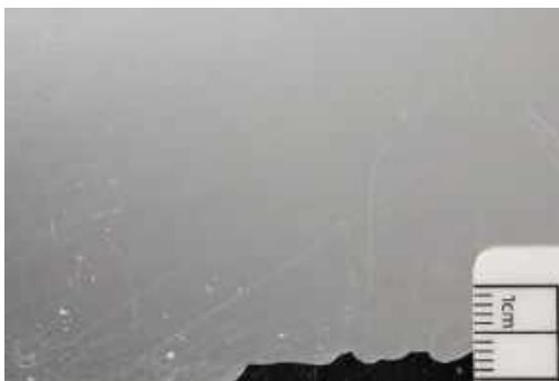
Figure 73 Presto aluminium-based. Mirror-finish surface, good adhesion. Radio-Genève, DY5107. Jeunesses musicales , May 1951.
