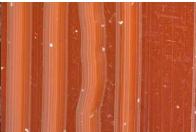
Gevaphone, Radio-Lausanne, 9341. Groove striations. USB micrograph, 250x. Reportage Théâtrale de Stella, 02 December 1942.
