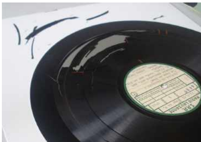
Thorens 1st period, Radio-Lausanne, 4486, 1941. Coating peeling away.
