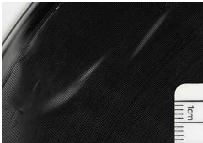
Simplat/Simplex, Radio-Lausanne, 300, 1937. Macrophotograph of flaking coating. Conversation with Blanche Richard, 27 December 1937.
