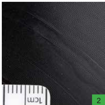
Coating flaking Slight flaking
