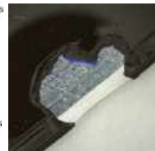
Pyral, DR4722, 1947. Bevelled aluminium edge, blue coating.
