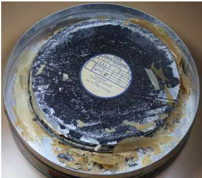
Figure 71 Inadequate storage in metal cans of 1945 Pyral zinc-based discs, resulting in cellulose nitrate decomposition. The greaseproof paper is shredded.
