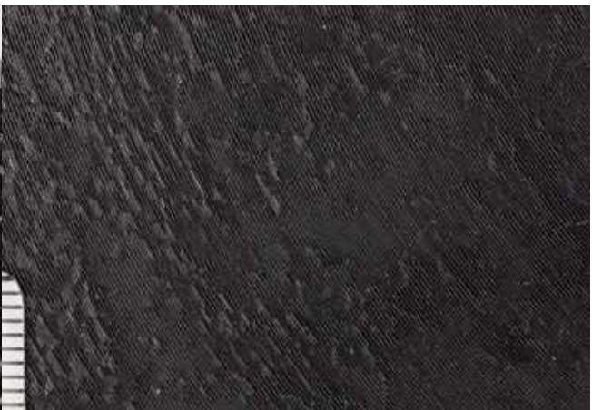
Pyral zinc-based, Radio-Lausanne, 181X, 1937. Macrophotograph of blisters and flaking coating. 25th anniversary of the Waldensian Scouts, scenic game , 6 June 1937.
