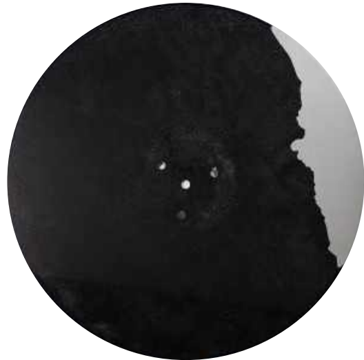
Presto Green Label, Radio-Genève, DY5107, 1951. Coating peeling away from the metallic substrate.
