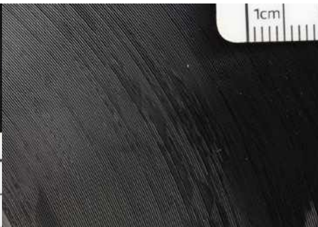
Simplat/Simplex, Radio-Lausanne, 8132, 1942. Macrophotograph of cracked and flaked coating. Visit to Salon romand du livre de Neuchâtel, 27 May 1942.
