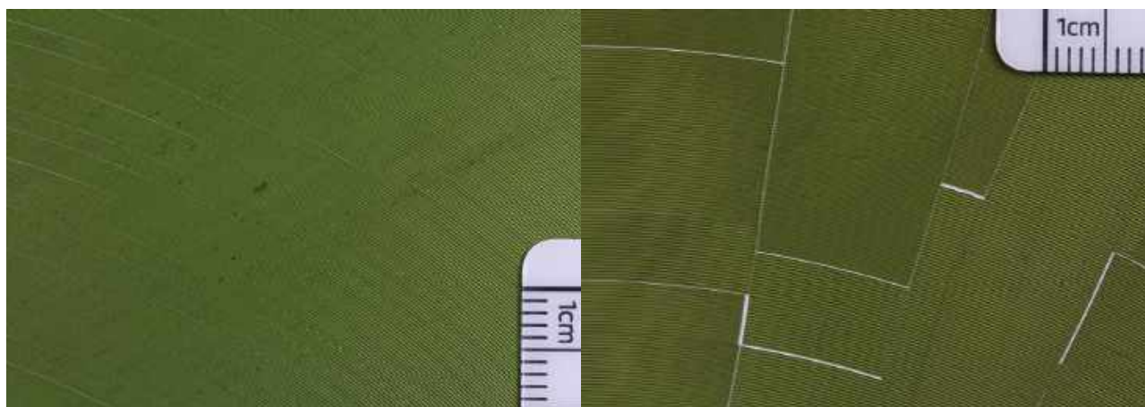
Thorens 3rd generation, green. Radio-Genève, DJ4700-5, 1947. Macrophotograph of a tangential crazing network.
