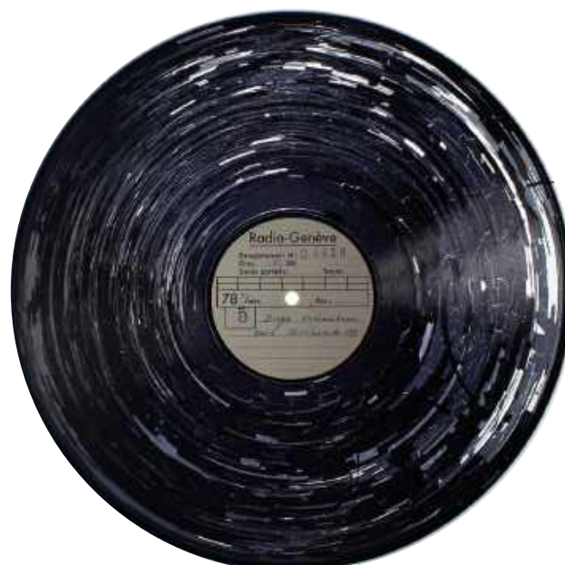
Simplat/Simplex, Radio-Genève, C4328, 1943. Gelatin coating peeling away. Bach Cantate 123 , by Diego Ochsbein, 6 October 1943.
