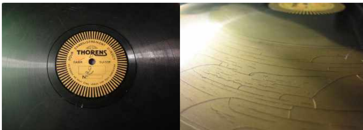
Thorens, 2nd generation disc (?). Right: dark green disc side. Left: dark green disc side with disc yellowing (photochemical degradation or excessive humidity?).
