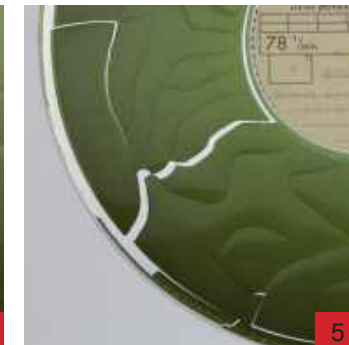
Coating flaking, large cracks
