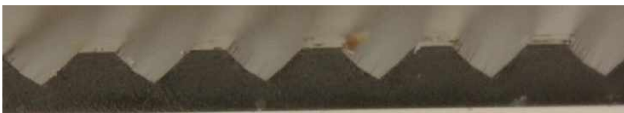
Gevaphone, Radio-Lausanne, 9341, 1942, Stratigraphy, cross-section. USB micrograph, 250x. Reportage Théâtrale de Stella, 02 December 1942.
