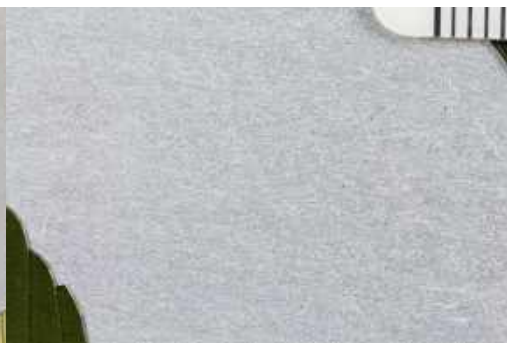
Figure 78 Thorens 3 rd generation, aluminium-based. Porous surface, poor adhesion. Radio-Lausanne, 22110, La chaîne du bonheur , 17 January 1947.
