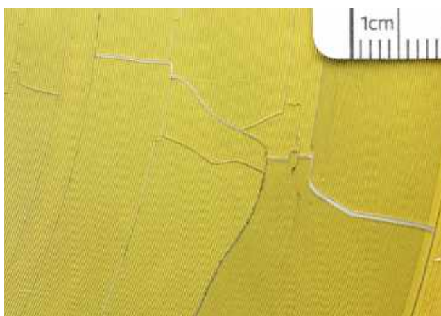
Thorens 3rd generation, yellow. Radio-Lausanne, 16634, 1945. Macrophotograph of a crazing network and cracked coating.
