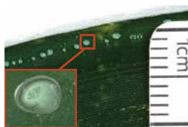
Small blisters air inclusion on the periphery of the disc
