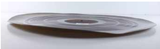
Decelith flexible, Radio-Genève, J230, 1941. Warped disc. Onze hommes, radiogame, 16 November 1941.
