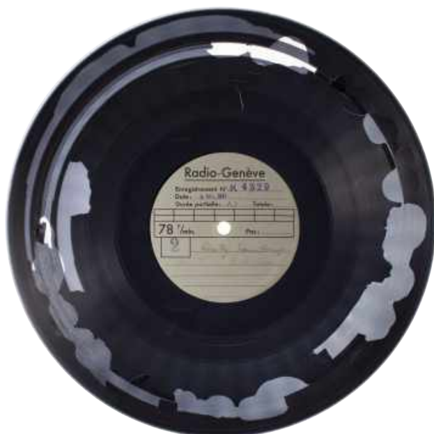
Simplat/Simplex, Radio-Genève, K4329, 1943. Gelatin coating peeling away. Roulez tambours , 6 November 1943.
