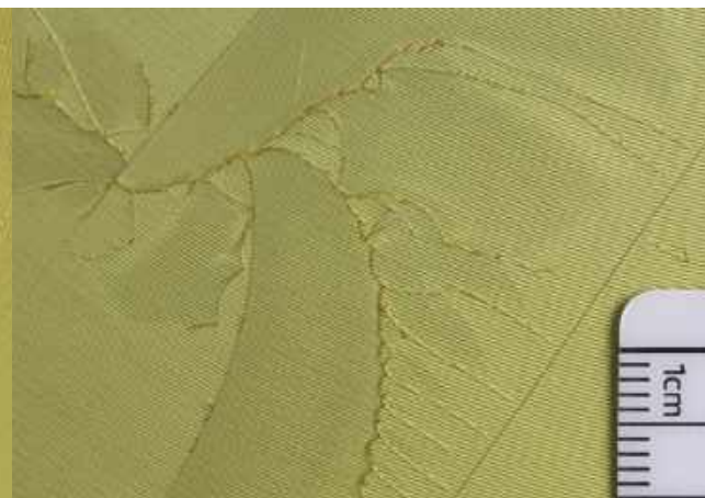
Thorens 2nd generation, Radio-Lausanne, 7498, 1942. Macro photograph of crazing, aluminium not visible. Choeur mixte de Moudon, 25 January 1942.
