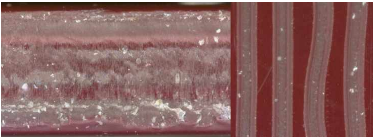
Decelith flexible, Radio-Lausanne, 7X, 1936. Right: Stratigraphy, cross section. Left: groove walls striations. USB micrograph, 250x
