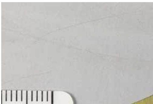
Figure 77 Thorens 2 nd generation, aluminium-based. Mirror-finish surface, good adhesion. Radio-Lausanne, 7399. Bon dimanche, radioplay , 19 February 1942.
