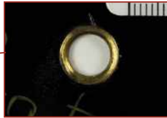
Central hole enclosed by a brass ferrule to strengthen the disc. Glass (1), metal ferrule (2), bevelled glass (3, 4) to facilitate). Detail of the Dutch patent NL 48190C, 1937
