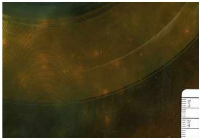
Pyral, black with green and amber hues, Radio-Lausanne, 30171, 1948. Discolouration of the coating (migration of the dye?). Interview Roberto Rossellini , by John Pasetti, September 1948.
