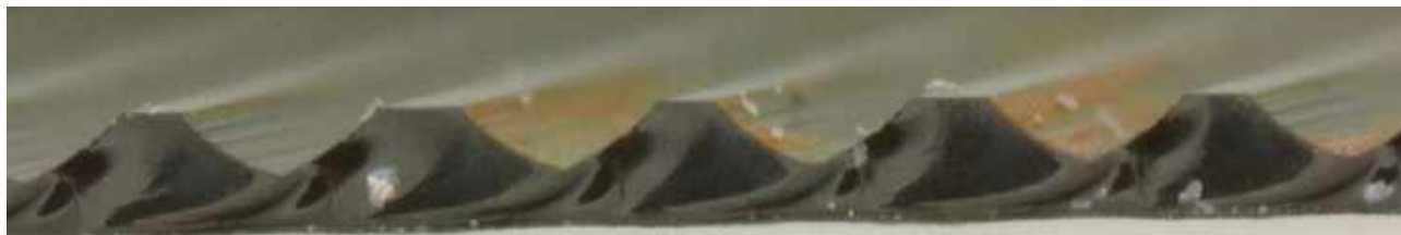
Thorens 1st period, Radio-Lausanne, 4486, 1941. Stratigraphy, cross-section. > 50% cutting depth. USB micrograph, 250x. Revue militaire du Régiment 2, Notre pays, 11 March 1941.
