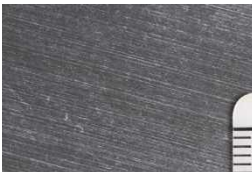
Figure 75 Pyral zinc-based. Lamination marks(?), poor adhesion. Radio-Lausanne, 150X, Banquet at the Livery-Club London , 31 May 1937.
