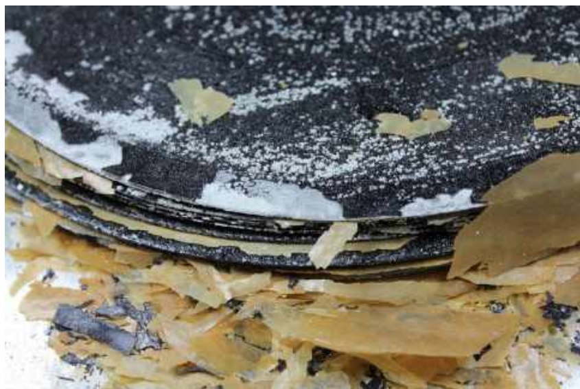
Figure 71 Inadequate storage in metal cans of 1945 Pyral zinc-based discs, resulting in cellulose nitrate decomposition. The greaseproof paper is shredded.
