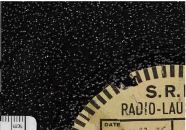
Pyral zinc-based, Radio-Lausanne, 22X, 1936. Macrophotograph of a coating with burst blisters. Switzerland-Italy match , April 1936.
