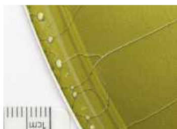
Small blisters air inclusion on the periphery of the disc
