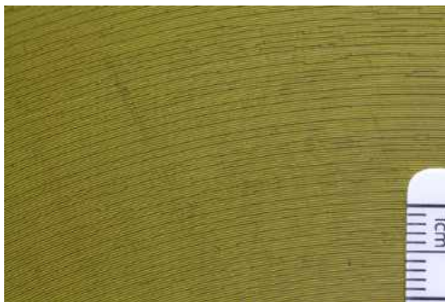
Thorens 3rd generation, yellow. Radio-Lausanne, 30911, 1948. Macrophotograph of a crazing network.
