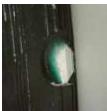
Pyral, 45105, no date. Bevelled aluminium edge, green coating
