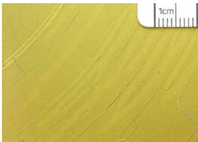
Thorens 3rd generation, yellow. Radio-Lausanne, 16634, 1945. Macrophotograph of a crazing network.
