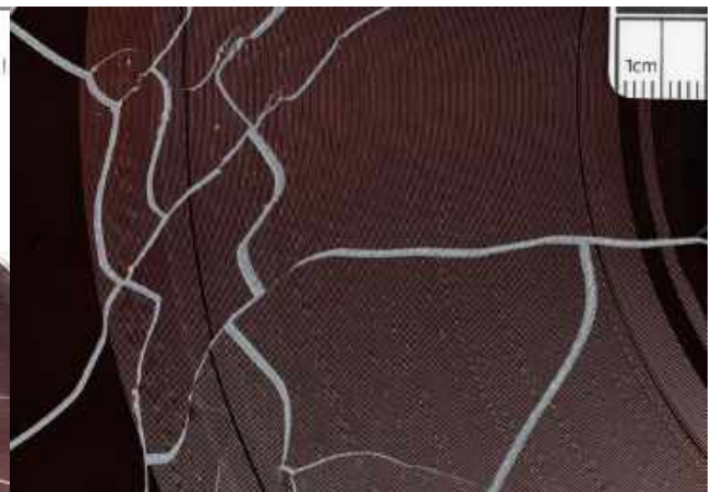
Pyral ersatz, Radio-Lausanne, 10945, 1943. Macrophotograph of large cracks.
