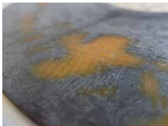
Figure 66. Discoloured coating and palmitic acid.
