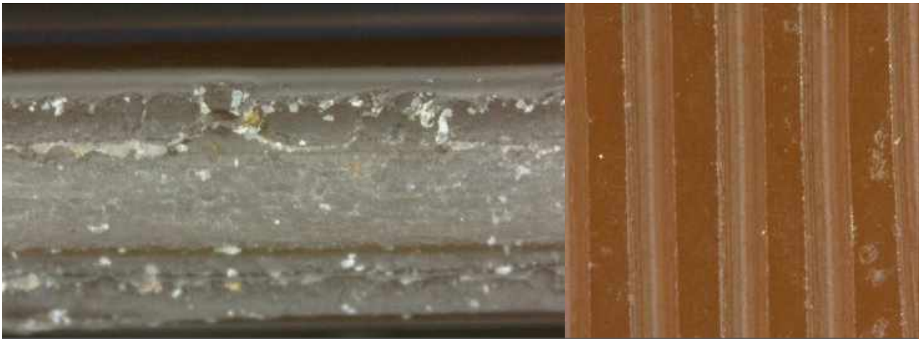
Decelith flexible, Radio-Genève, L232, 1941. Right: Stratigraphy, cross-section. Left: groove walls striations. USB micrograph, 250x
