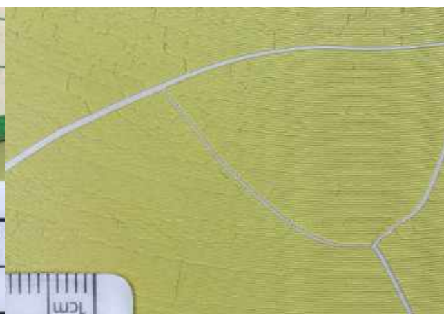
Thorens 2nd generation, Radio-Lausanne, 325C, 1942. Macro photograph of large cracks and crazing. Aluminium substrate visible. Corsier-sur-Vevey bells, 14 May 1942.
