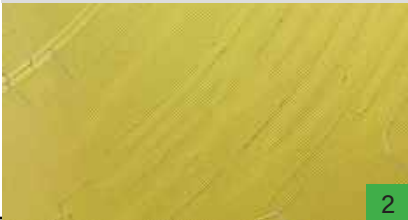
Cracked (tangential to the groove)
