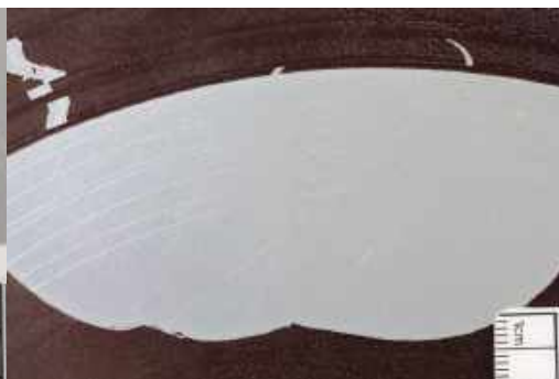
Figure 74 Pyral ersatz aluminium-based. Mirror-finish surface, good adhesion. Radio-Lausanne, 13674. Stettler-Ackermann, Loch Lomond , 16.11.1944.
