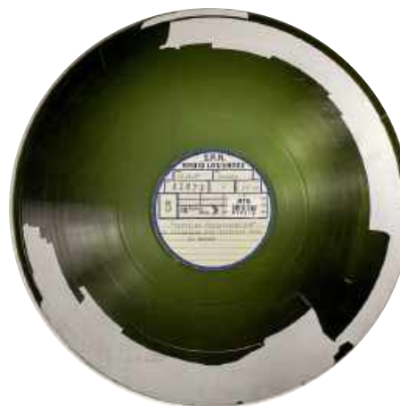
Thorens 3rd generation, dark green. Radio-Lausanne, 23677, 1947. Coating peeling away.
