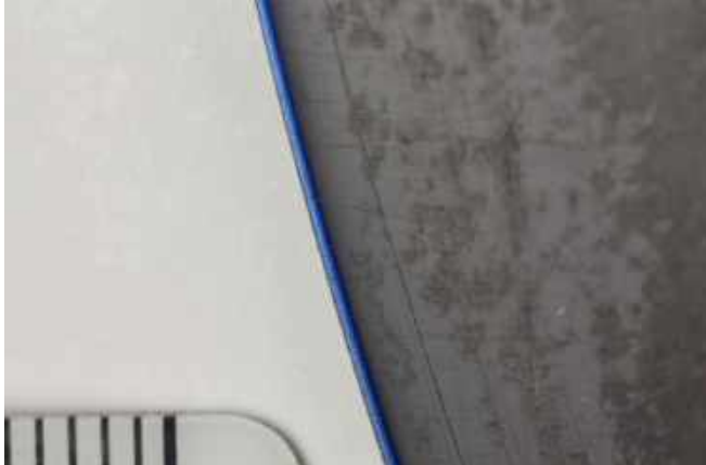
Presto Green Label, Radio-Genève, DY5107-5, 1951. Macro photograph of palmitic acid layer.
