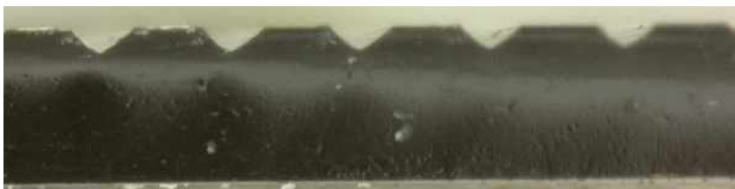
Thorens 3rd generation green, Radio-Genève, DW4621, 1946. Stratigraphy, cross-section. V-shaped cut. USB micrograph, 250X. Report on Princess Juliana's Arrival: Red Cross for Holland, 23 May 1946.
