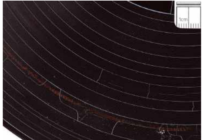
Pyral ersatz dark red, Radio-Genève, Q280, 1942. Crazing network. La Quinzaine sonore , 14 August 1942.
