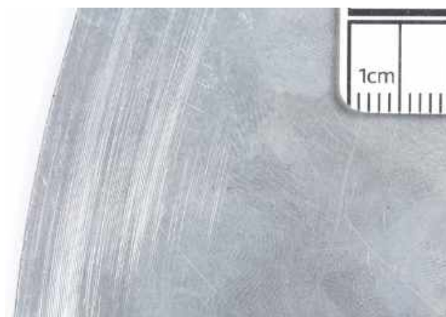
Thorens 1st period, Radio-Lausanne, 4386, 1941. Macro photograph of uncoated aluminium, circular striations caused by the playback on the turntable (?), fingerprints.
