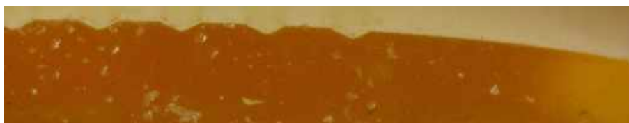
Thorens 2nd generation, Radio-Lausanne, 7399, 1942. Stratigraphy, cross section. USB micrograph, 200x. Curved effect on the periphery of the disc. Bon dimanche, radio theatre , 19 February 1942.
