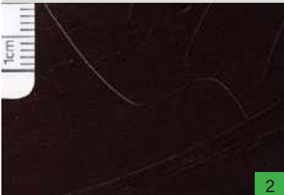
Cracked (perpendicular to the groove)
