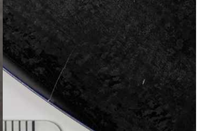
Presto Green Label, Radio-Genève, DY5107-6, 1951. Macro photograph of thin cracks, light palmitic acid layer.
