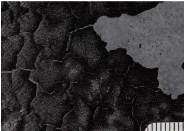
Pyral zinc-based, Radio-Lausanne, 22X, 1936. Macrophotograph of flaking coating, zinc corrosion and palmitic acid layer. Interview Ott (gliding) , by Cl. Schubiger, 11 September 1936.
