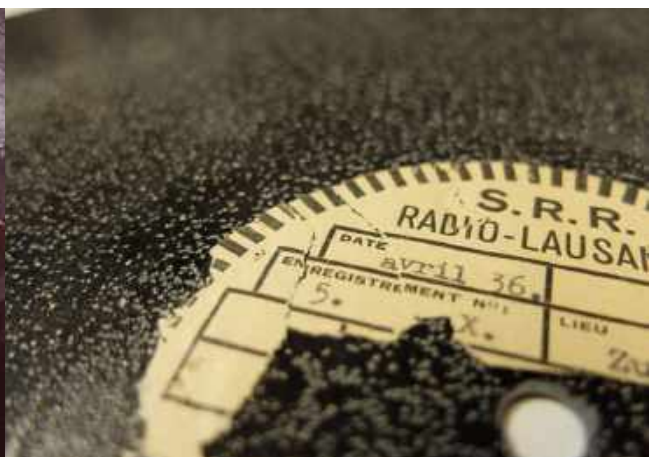
Pyral zinc-based, Radio-Lausanne, 5X, 1936. Coating with burst blisters. Switzerland-Italy match, April 1936.
