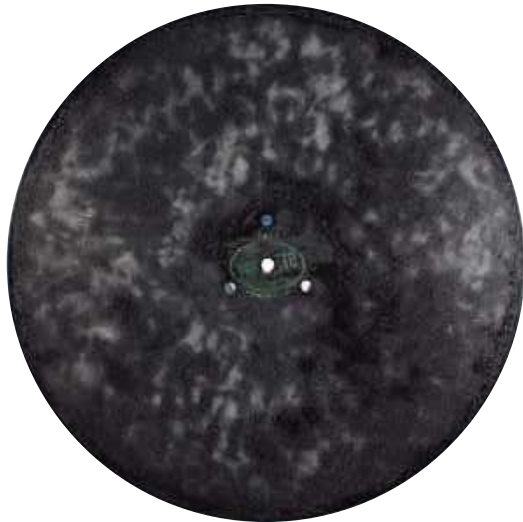
Presto Green Label, Radio-Genève, DY5107, 1951. Palmitic acid layer.
