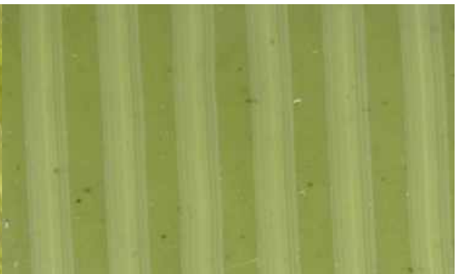
Thorens 3rd generation green, Radio-Genève, DW4621, 1946. Groove side, walls striations. USB micrograph, 250X. Report on Princess Juliana's Arrival: Red Cross for Holland, 23 May 1946.
