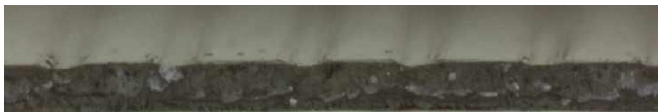
Simplat/Simplex, Radio-Lausanne, unknown accession number. Stratigraphy, cross-section. U-shaped. Very shallow cut. USB micrograph, 250x.
