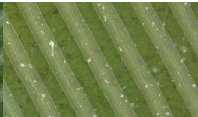
Thorens 3rd generation striations dark green, Radio-Lausanne, 41100, 1947. Groove walls striations and dust. USB micrograph, 250x. Indian folklore, 1947.
