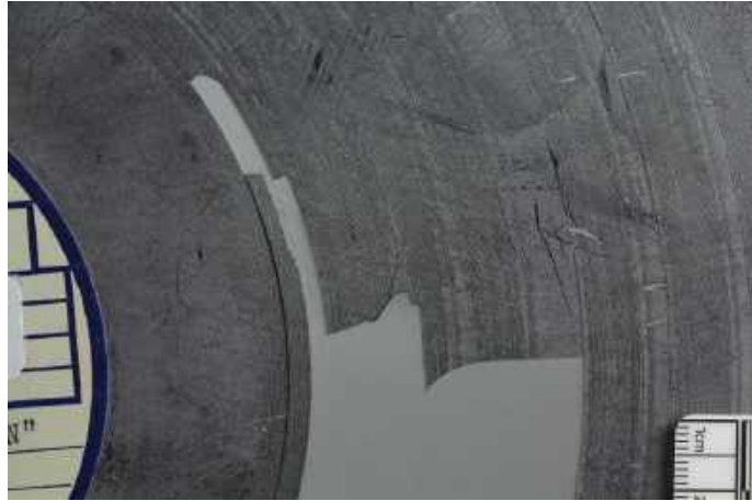
Figure 70 Plasticiser loss. Palmitic acid and peeling of the coating.
