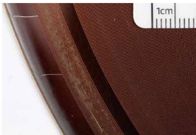
MSS, Radio-Genève, DS5100, 1951. Crazing, macrophotograph. La vie parisienne , operetta of Jacques Offenbach, 6 January 1951.
