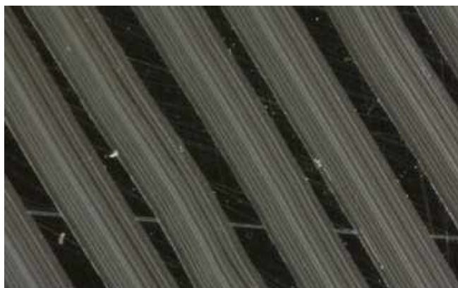
Thorens 1st period, Radio-Lausanne, 4386, 1941. Wide cutting depth and groove walls striations. USB micrograph, 250x. Les Compagnons de la Chanson, 8 March 1941.
