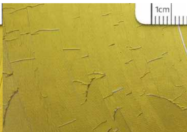
Thorens 3rd generation, yellow. Radio-Lausanne, 16634, 1945. A network of cracks, radial and tangential to the groove.
