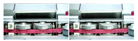
**FIGURE 3.** Test for video shooting. On the left, a correct setting of the camera: each frame is clear and the text is readable. On the right, a wrong setting of the camera. The aim is to detect physical defects of the tape (due to aging or joints) that may correspond to a specific noise in the audio signal. Audio is directly recorded from a secondary output of the STUDER A810.
