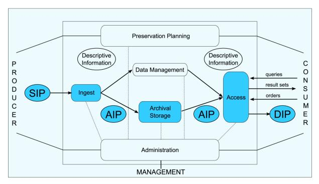
**Fig.2** OAIS Schema with marked workflow of the Information packages SIP, AIP and DIP: ingest, storage and access.
