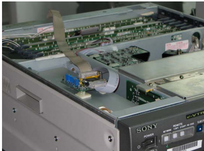
Figure 8 RAI QC board mounted inside MSW-2000
