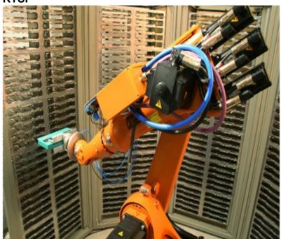
This project uses a robot to automate tape handling.
